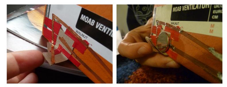
Pro tip: Your battery holder should be in a location that will allow you to clamp it shut on the battery with a binder clip. (I forgot to do this!)
