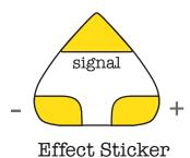
The effect sticker has three pads: + and - for power and a signal pad that generates the pattern.
