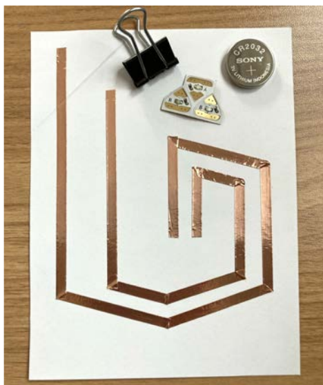
Conductive copper tape, LED Circuit Stickers, 3 volt "coin cell" battery, small binder clip
