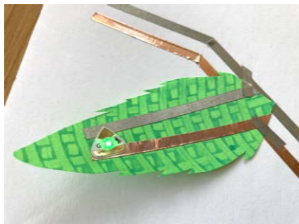
Small pieces of conductive fabric tape placed on top connect corresponding traces
