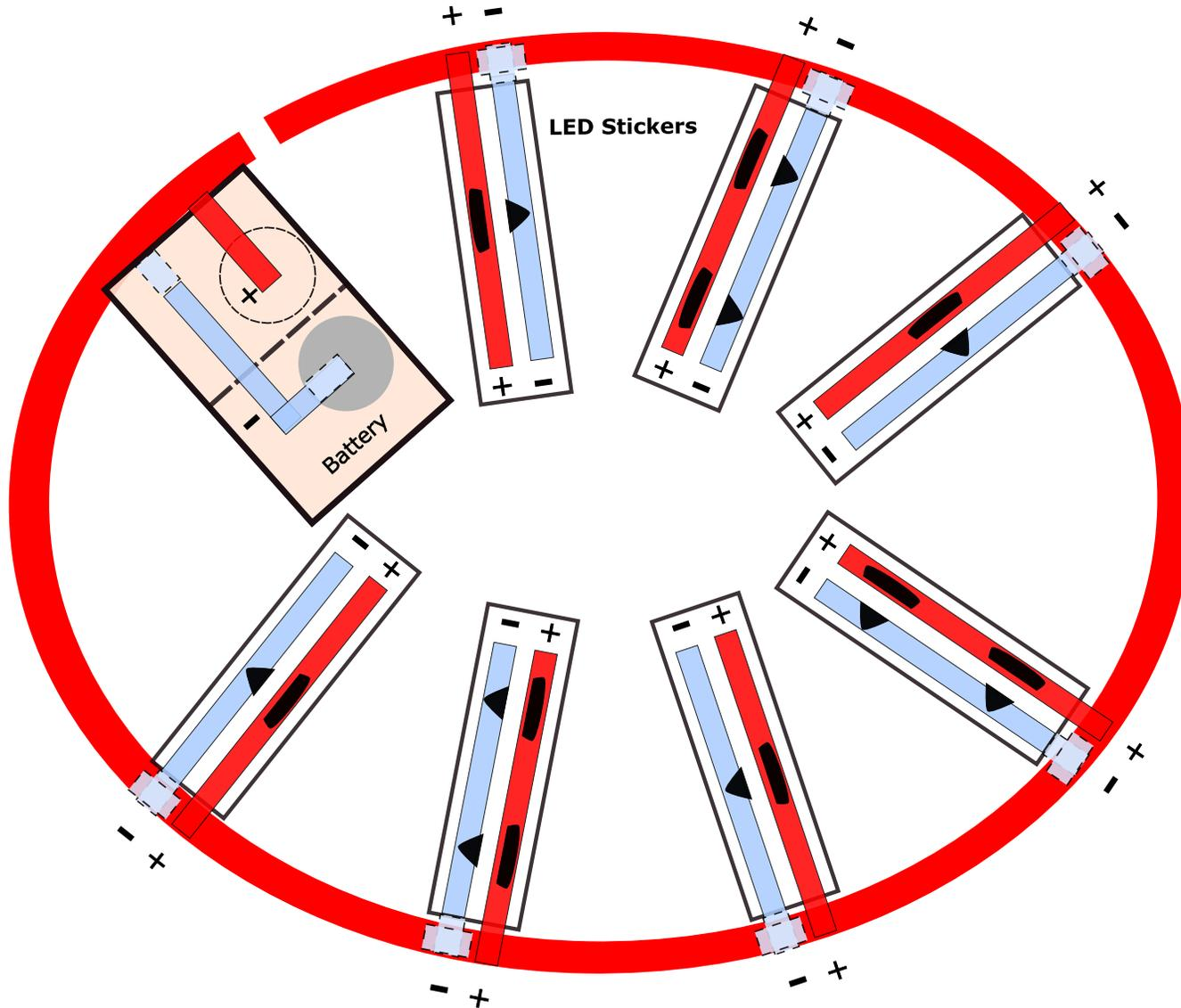
To create the power & ground rail for your Paper Circuit Chandelier, apply the positive lead to the front side of a 1/4" wide ribbon and the negative lead to the back side. You may add as many LED flags to your branching circuit as you wish.
