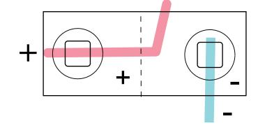
Inside view of battery holder with flat magnets
