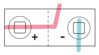
Inside view of battery holder with flat magnets placed under conductive fabric tape traces
