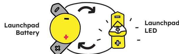
power from the battery flows through the LED light, causing it to shine. This continuous loop is called a complete circuit.
